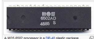
A MOS 6502 processor in a DIP-40 plastic package.
