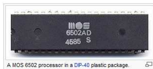
A MOS 6502 processor in a DIP-40 plastic package.
